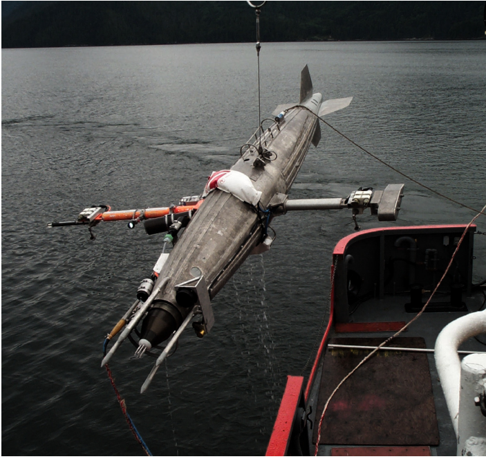
Figure 2: The Towed Ocean Microstructure Instrument (TOMI) developed by Rolf Lueck at the University of Victoria. Here it is being recovered from the water in Knight Inlet after making simultaneous measurements of the turbulent small-scale fluctuations of velocity and temperature, as well as measuring the backscatter of high-frequency sound from biological organisms and the turbulence. The masts at right angles to the main body of the instrument contain other sensors and become vertical in the water, with the orange one on top.
